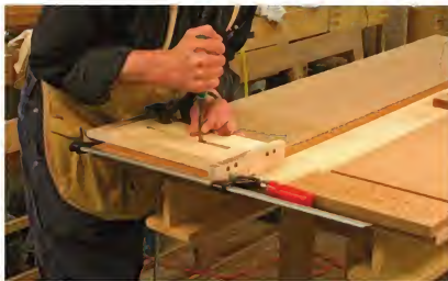
Double duty. After routing, the mortising jig also serves as a guide for the chisel to square the corners of the through-mortises.
